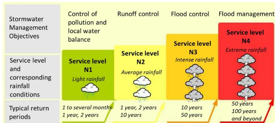
*Figure 1 Stormwater management objectives and choice of precipitation return period for the design of hydraulic structures (adapted from DGALN, Cerema – Rejets d'eaux pluviales Principes généraux, 2014)*
